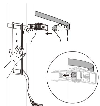
Ask a second person to wrap the strap around the column. Person #2 should insert free end of strap into the slot of the ratchet buckle.
