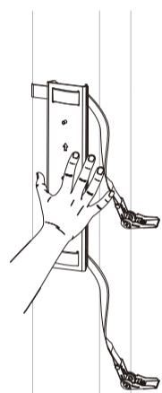
Hold column mounting bracket to the column where you would like to mount the TV.
